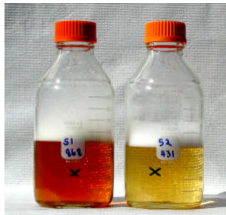
Figure 10. Prepared samples before filtration, Left – Surge 1 Out, 868 mg/L, Right – Surge 2 Out, 431 mg/L. “X” is drawn on the back side of the 1 liter bottles to demonstrate sample clarity.
