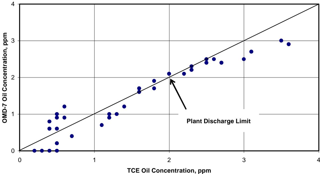
Figure 9. Comparison of OMD-7 and TCE dispersed oil results.
