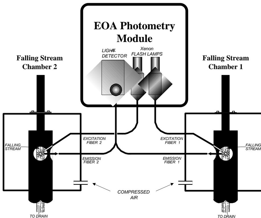
Figure 2. Schematic diagram of the EOA System.
