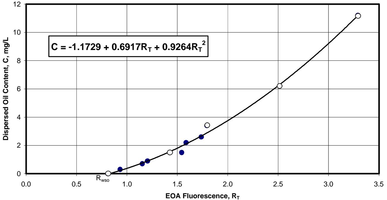
Figure 5. EOA calibration curve – FC-5, produced water.
