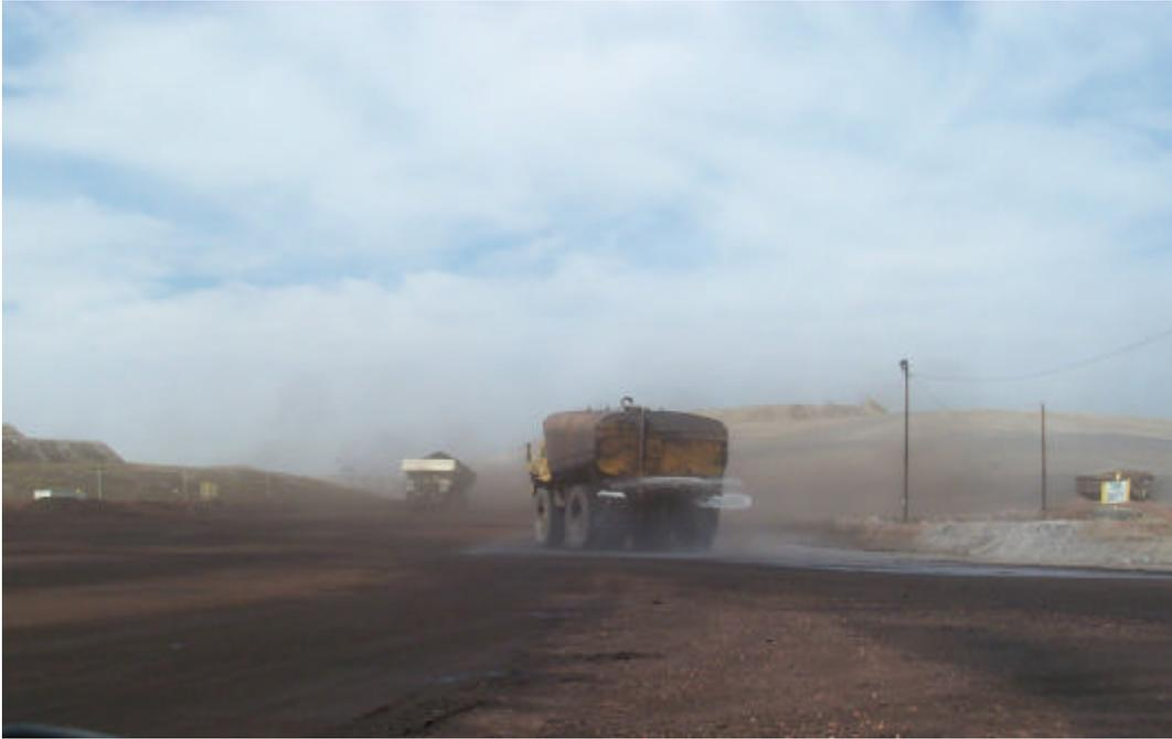
**Figure 2: 44,000 Gallon Water Truck in Operation in Coal Hopper Area During Windy Day.**
