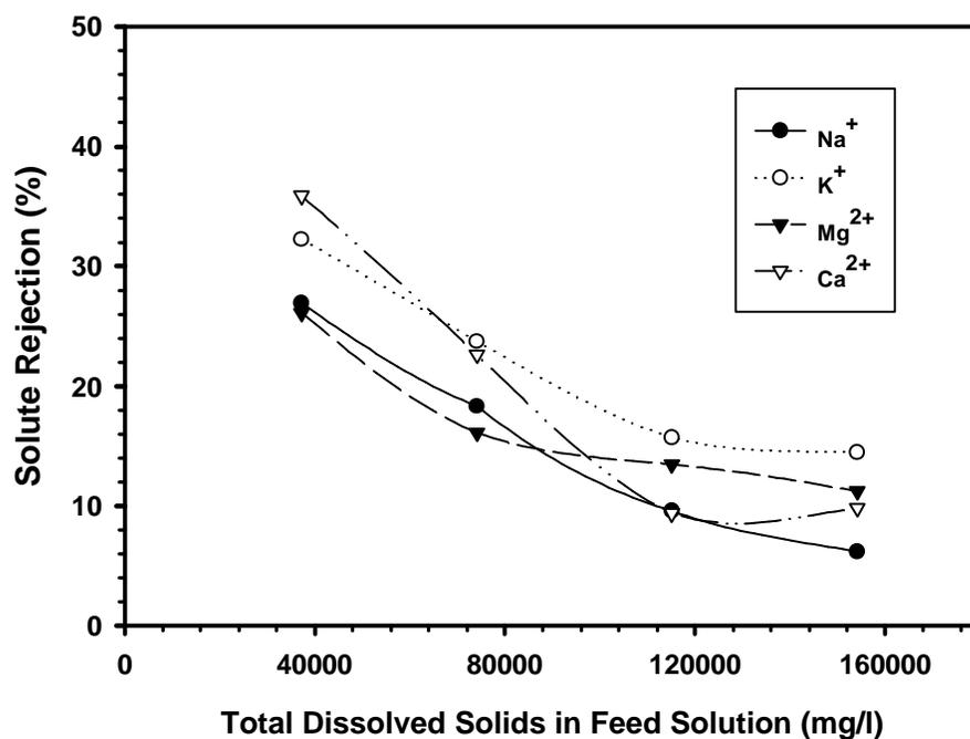
Figure 4. Solute rejection of cat ion as a function of TDS (membrane compacted to 36.1Mpa) for produced water.
