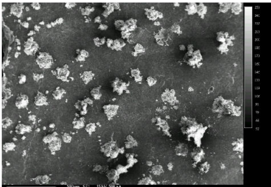
Figure 5. Microprobe scan showing distribution of NaCl crystals.
