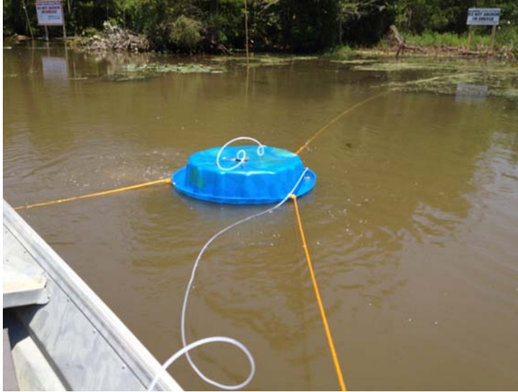
Figure 7 – Methane Sampling Device Using a Swimming Pool and Tubing
