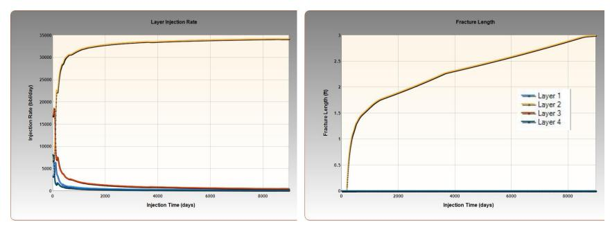
Once the first fracture opens up, the fractured layer (2) takes nearly all the flow.
