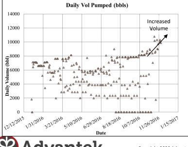
An increase in injection rate and total batch size allowed for better solids distribution within the fracture and results in lower fracture closure pressure / stress accumulation per batch.
