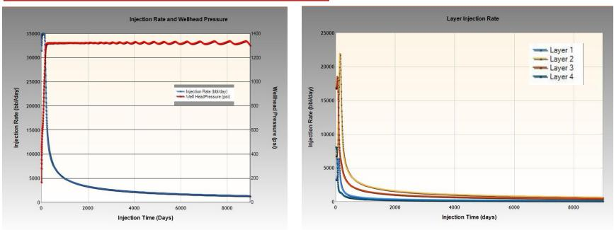
With the surface pressure restricted, the total flow rate decreases as the damage builds, then increases again as an open fracture reduces the restriction
