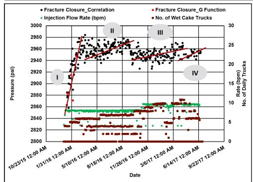
Operating parameters (injection rate, daily injection duration, weekly rest time) have a strong impact on total formation capacity
