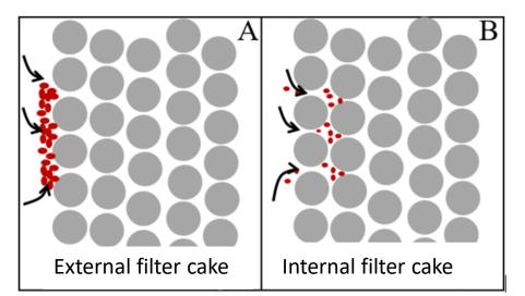
Wellbore damage is a function of solids content, particle size, pore throat size, and fracturing strategy
