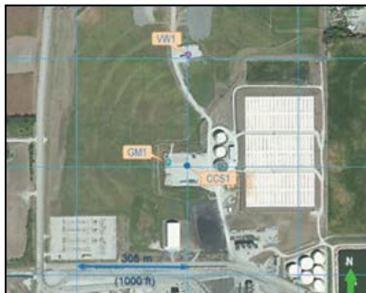
FIGURE C.9. Map of well locations (below) and diagram (right) for vertical arrays showing configuration of borehole and monitoring equipment for the IBDP site in relation to stratigraphy: the WellWatcher PS3 geophone array in the CCS1 well; the OYO, three-component, 31-level array in the GM1 well; and the Westbay system in the VW1 well for sampling and pressures readings at 11 levels. Source: from Will et al. 2014.
