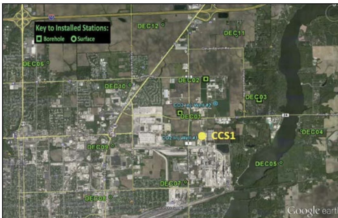
FIGURE C.10. Map of USGS surface seismograph stations. CCS1 is the injection borehole; the three “borehole” installations shown are 500 feet deep. Source: Hickman et al. 2014.
