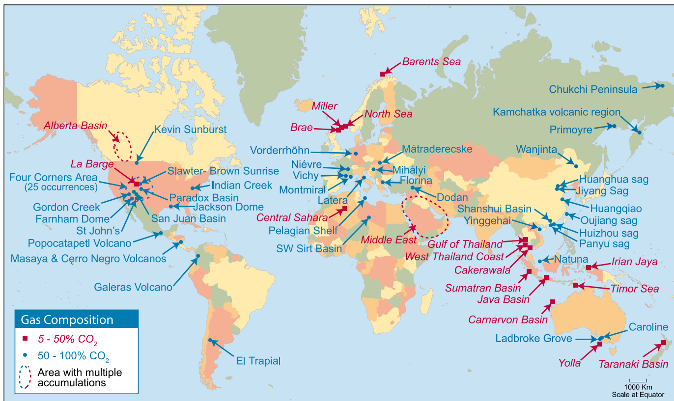
Figure 5.11 Examples of natural accumulations of CO 2 around the world. Regions containing many occurrences are enclosed by a dashed line. Natural accumulations can be useful as analogues for certain aspects of storage and for assessing the environmental impacts of leakage. Data quality is variable and the apparent absence of accumulations in South America, southern Africa and central and northern Asia is probably more a reflection of lack of data than a lack of CO 2 accumulations.
