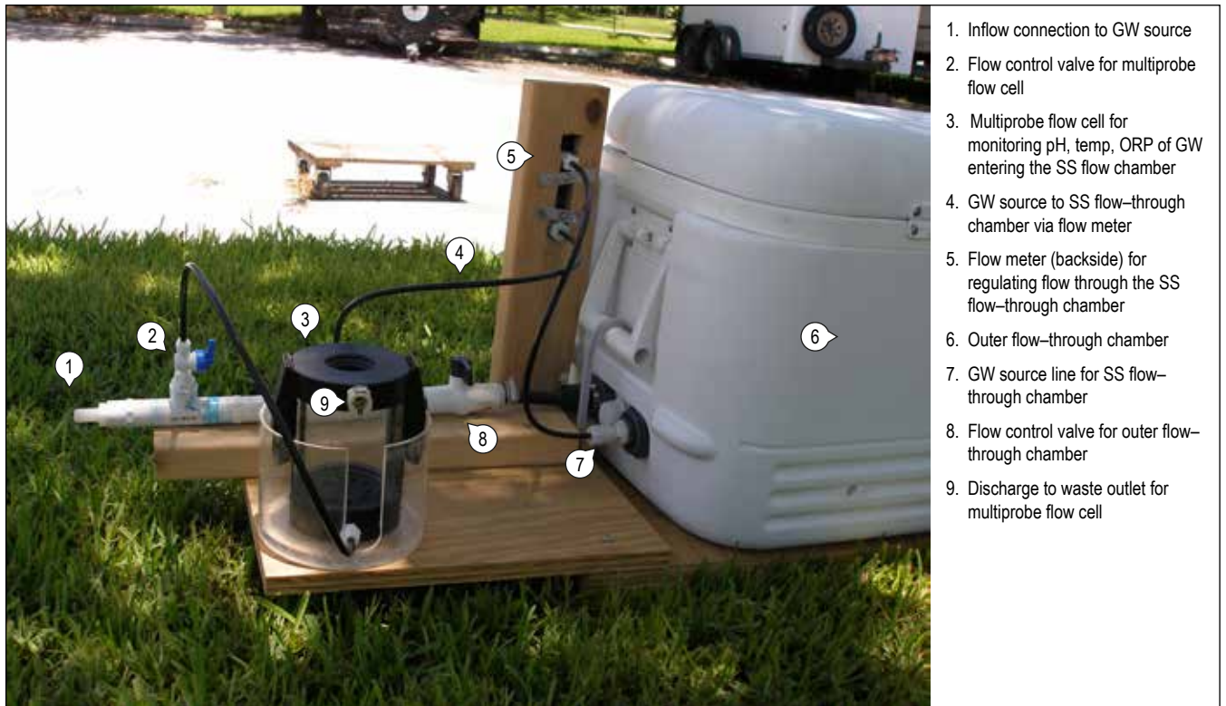
Figure 1-11. The outer flow-through chamber flow rate controls and multiprobe attachment fittings (rear view).
