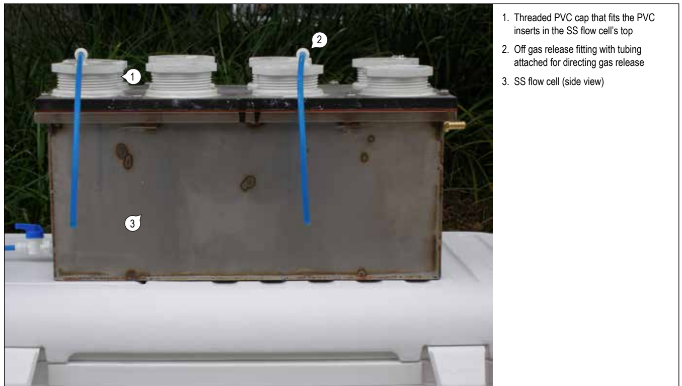
Figure 1-9. The complete stainless steel flow-through chamber with diffusion chambers inserted (side view).
