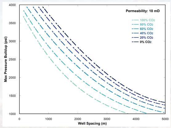
As system compressibility (Ct) increases, pressure buildup decreases. CO2 is approximately twice as compressible as N2 at reservoir conditions.
