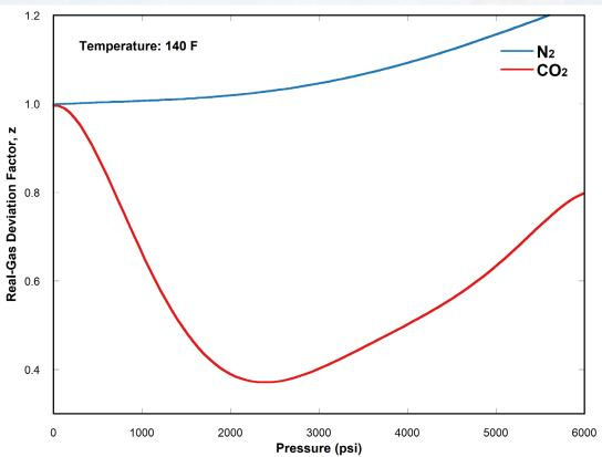
Binary mixture's Z-factor decreases at initial reservoir pressure as flue gas composition shifts from 100% N2 to 100% CO2, also shifting fluid compressibility
